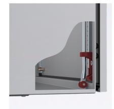
A further improvement is that the plastic holders which guide the rods have a new geometry which puts the door in the right position during closing. This guarantees that the sealing between the door gasket and the enclosure rain gutter is perfect, even in applications in which the door is heavily loaded and may tend to hanging. The gasket compression is improved and any risk of the door not closing completely is avoided.
