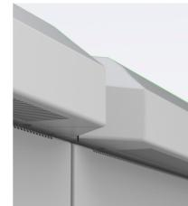
The walls of the enclosures in the floor standing aluminium range are made from high quality marine grade aluminium, AIMg3, which is light and highly corrosion resistant. This material also offers good heat dissipation and the double wall design provides 80% higher cooling efficiency than a single wall version, if the enclosure is installed outdoors and exposed to the sun.
