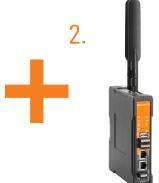
Security/NAT/VPN/U-link Router, Fast Ethernet, 2x RJ45 10/100/1000BaseT(X)
