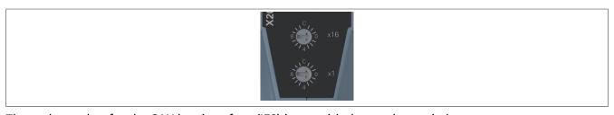
The node number for the CAN bus interface (IF2) is set with the two hex switches.
