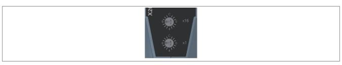
The node number for the CAN bus interfaces is set with the two hex switches.
