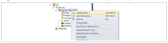
• Slave module X20IF10G3-1 can now be selected; it is marked as "CIFX RE/ECS" in a 3rd-party environment. The module is attached to the master with "OK".
