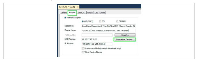
• Now select the Ethernet interface – which is intended to act as an EtherCAT connection and is connected to the EtherCAT slave (X20IF10G3-1) – and confirm by clicking "Install". The connection is established by clicking on "Search".
