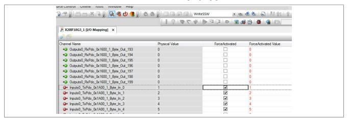
• The input data in the TwinCAT environment can be read for verification. To do so, double-click on TxPDO (input data) of the EtherCAT slave to open it. The input data can be read in column "Online".
