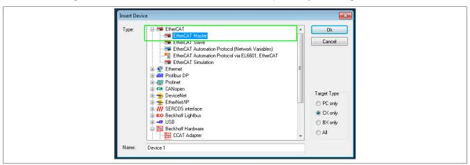
• The master configuration is opened by double-clicking on the added "Device 1".
