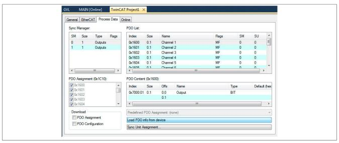
• The configuration can be transferred to the module with button "Activate configuration".
