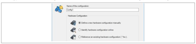
• If "Define a new hardware configuration manually" was selected, the hardware is selected in the next step. In order to simplify the search, different filters can be set for this in the Hardware Catalog. Finally, the Automation Studio project is created by selecting the required hardware is and clicking "Finish".
