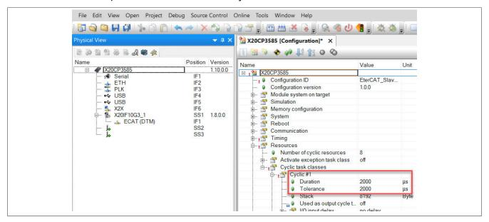
• Adjust "Data exchange time" on the EtherCAT slave to the system cycle time (X2X Link or POWERLINK), enable timer synchronization and "Manual start of bus communication".
