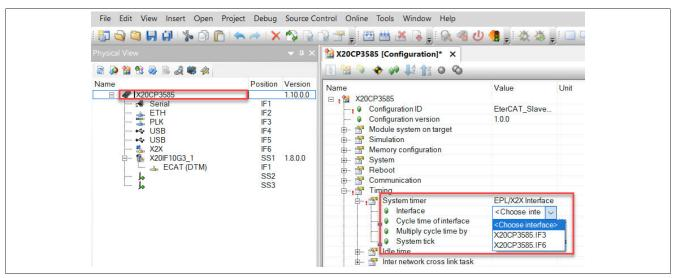
• The optimal response time is achieved if the application is running in task class Cyclic#1 and the cycle time of the task class corresponds to the EtherCAT bus cycle time.
