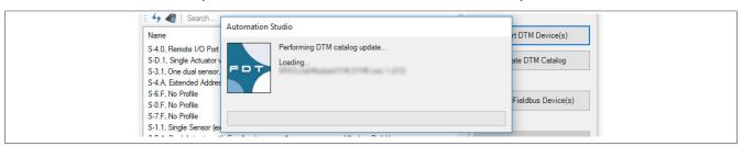
• Click on "EIP(DTM)" on EtherNet/IP scanner (master) X20IF10D1-1, drag the EDS file from the Hardware Catalog and attach it to the EtherNet/IP scanner (master).
