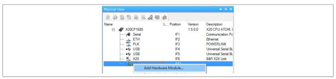
• The module is added to the project via drag-and-drop or by double-clicking on the interface card.
