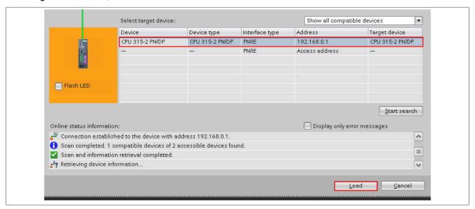
• Before loading, a notification window opens and lists a preview of all loading processes. This can be used to check whether the correct data is being transferred. The data is transferred after pressing **Load**.
