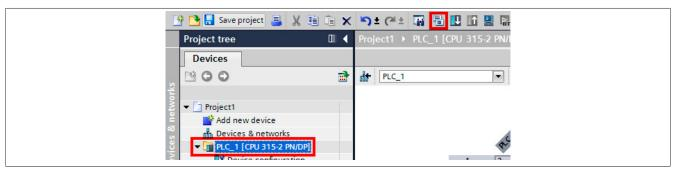
• After the project has been successfully compiled, it can be loaded onto the device. To do this, select button **Download to device** in the toolbar.
