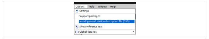
• The downloaded description file is selected in the dialog box and added to the project with button **Install**. This adds the interface module to the Hardware Catalog of the TIA portal.
