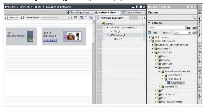
• The installed controller and the interface module are connected via PROFIBUS. For this purpose, the PROFIBUS interface of the controller is connected to the PROFIBUS interface of the interface module via drag-and-drop.
