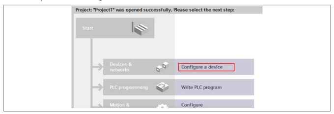
• The controller used is selected using Add new device and added to the configuration with button Add.
