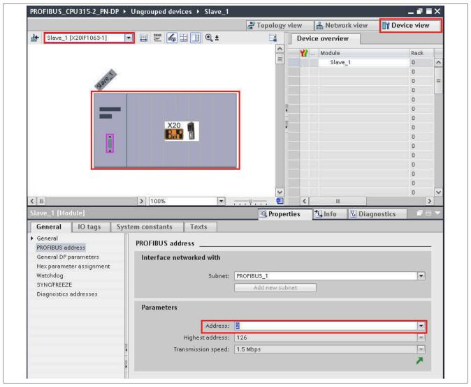
In addition, further configurations can be carried out for the module. All set parameters must match the settings in Automation Studio.
