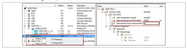
• "Start of bus communication" must be set to "Controlled by application".
