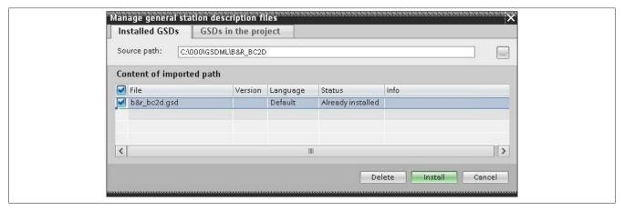
• Now the installed interface module can be used in the project. The interface module is selected in the Hardware Catalog and then dragged and dropped into the project.
