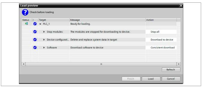
• The result of the loading process is listed and must be confirmed with Finish.
