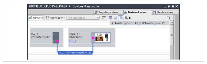
• To establish the communication between PROFIBUS master and PROFIBUS slave, the PROFIBUS address of the slave must be set. This must match the set PROFIBUS address of the interface module in Automation Studio.
