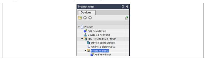
• If a new program is created using **Add new block**, the name of the block and the programming language are first set and confirmed with **OK**.
