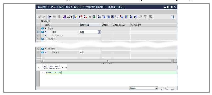
• A **tag** can now be created in the application to link the variable to an output via an address. This is created with "%QB + Address" or "%IB + Address":
