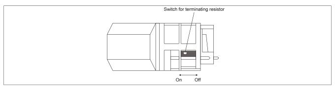
A terminating resistor is integrated in the interface module. It can be switched on or off with a switch on the bottom of the housing. A switched-on terminating resistor is indicated by LED "TERM".
