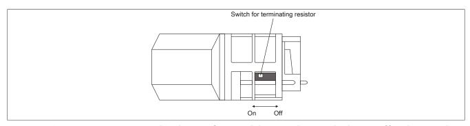
A terminating resistor is integrated in the interface module. It can be switched on or off with a switch on the bottom of the housing. A switched-on terminating resistor is indicated by LED "TERM".
