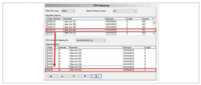
• TPDOs are edited by changing to "TPDO" under "Filter PDO type". Bytes that are not required can be removed from the assignment. This is done by selecting the relevant TPDOs and cutting the superfluous objects using the scissors.
