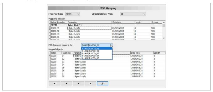
By default, the PDOs are filled with bytes. No change must therefore be made for the input bytes.
