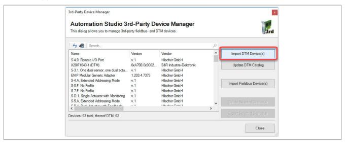
• Select the EDS file to be imported and confirm with OK. The EDS file is imported into Automation Studio.
