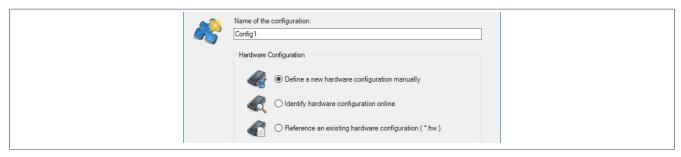
• If "Define a new hardware configuration manually" was selected, the hardware is selected in the next step. In order to simplify the search, different filters can be set for this in the Hardware Catalog. Finally, the Automation Studio project is created by selecting the required hardware is and clicking "Finish".
