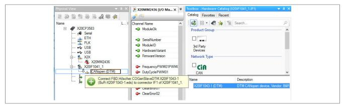
• Right-click on the device description file and select "Device configuration" to open the configuration environment for the EDS file.
