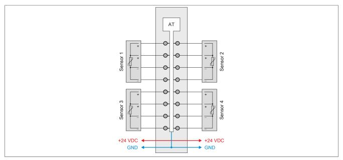
To guarantee accuracy, modules with a power dissipation <1.2 W must be connected to the left and right of this module.
