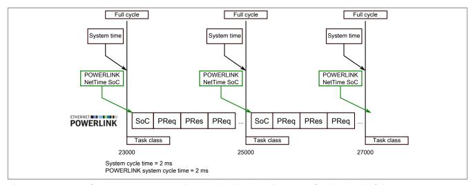
The POWERLINK reference time point is always calculated at the start of cycle (SoC) of the POWERLINK network. The SoC starts 20 µs after the system clock due to the system. This results in the following difference between the system time and the POWERLINK reference time:
