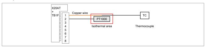
The thermocouple provides  $V(_{\Delta T})$  between the end of the thermocouple and the transition to the copper wire.
