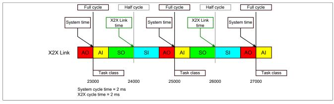
The reference time point on the X2X Link network is always calculated at the half cycle of the X2X Link cycle. This results in a difference between the system time and the X2X Link reference time point when the reference time is read out.
