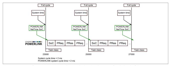
The POWERLINK reference time point is always calculated at the start of cycle (SoC) of the POWERLINK network. The SoC starts  $20 \,\mu s$  after the system clock due to the system. This results in the following difference between the system time and the POWERLINK reference time:
