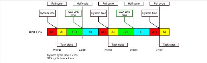
The reference time point on the X2X Link network is always calculated at the half cycle of the X2X Link cycle. This results in a difference between the system time and the X2X Link reference time point when the reference time is read out.
