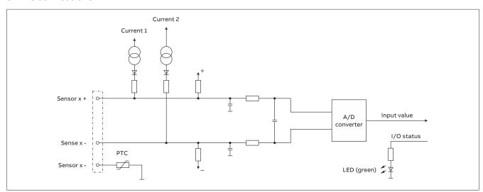
The following is an example of the assignment of the signals to the terminal connections of channel 1.
