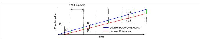
At startup, the internal counters for the controller/POWERLINK (1) and the I/O module (2) start at different times and increase the values with microsecond resolution.
