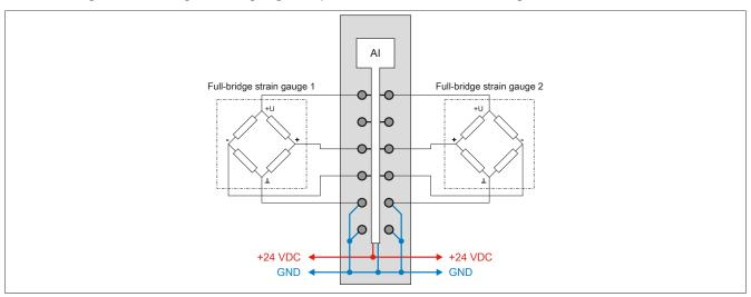
When connecting 3 or more full-bridge strain gauges in parallel, 2 lines must be connected together in an X20 terminal block.
