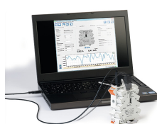
Configuration via WAGO Interface Configuration Software
