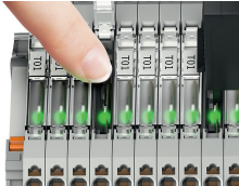
Configuration via push/slide switch
