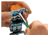
Terminal strip with mounting flanges Screwing a mounting foot (209-123). (Distance between mounting feet: approx. 25 ... 30 mm)
