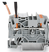
Insert fine-stranded conductors via operating tool.
