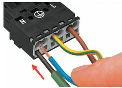
To terminate fine-stranded conductors, open the clamping unit via screwdriver (2.5 mm blade width) and insert a stripped conductor until it hits the backstop.
