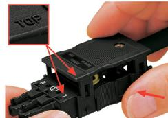
Latch the strain relief housing onto the plug/socket. Note the "TOP" inscription.
