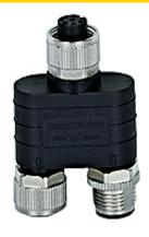
Plug-in connector, Y-adapter, IP67, M12 male connector (X2, evaluation device/previous plug-in connector), 8-pin, A-coded on M12 female connector (X3, sensor), 8-pin, A-coded and M12 female connector (X1, sensor/next plug-in connector), 8-pin, A-coded, for connection for including the PSENcode in the series connection of PSENmlock, when using SDD, corresponding to the used PSENcode type, use a different Y-adapter: 540315, 540316, 540337, 540338 (not 570489!).
