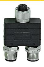
Plug-in connector, Y-adapter, IP67, M12 male connector (X1, evaluationdevice), 8-pin, A-coded on M12 female connector (X3, sensor), 5-pin, A-coded and M12 male connector (X2, evaluation device), 5-pin, A-coded, to conduct the OSSD signals from PSENmlock to an M12-port of PDP67.
