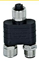
Plug-in connector, Y-adapter, IP67, M12 male connector (X1, evaluationdevice), 8-pin, A-coded on M12 female connector (X2, sensor) 12-pin, A-coded and M12 female connector (X3, sensor/next plug-in connector), 8- pin, A-coded, to connect PSENslock in series.
