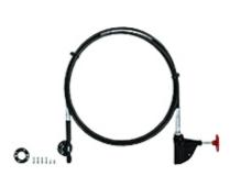
Push/pull cable release for the safety gate system PSENmlock, cable length 0.75m, package content = Push/pull cable and operator element. Ensure that this version is installed as straight as possible. With the escape releases with order no. 570466 and 570467 bending the push-pull cable can reduce the functionality and the service life.
