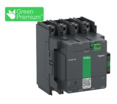
High power contactor, TeSys Giga, 4 pole (4NO), AC-1 <=440V 305A, standard version, 100...250V wide band AC/DC coil
