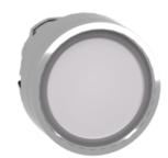
Head for illuminated push button, Harmony XB4, metal, white flush, 22mm, universal LED, spring return, plan lens
