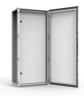
**Description:** Inner door provides a hinged mounting surface for equipment behind a standard or glazed front door. A mounting space of 80 mm, is available between the doors when the inner door is in the most forward position. Can be adjusted in depth by steps of 25 mm. The mounting plate remains usable behind the inner door. The door is equipped with two double-bit 3 mm locks.
