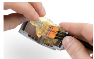
Simply extend the circuit: Open the gelbox, remove gel from the connector, open the connector and connect new components to the cable.
