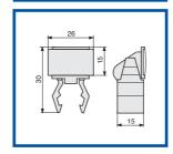
DUCTAMARK is mounted by snapping it onto the sidewall finger segments taking care that it is placed above the wires coming out to the sidewall slots.
