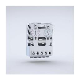
**Description:** Device with two independent thermostats, unlike thermostats with changeover contacts, connected devices can be switched in different temperature ranges. One thermostat with a normally closed contact for regulating heaters, and one with a normally opened contact for regulating cooling devices or signal devices. Sensor element thermostatic bimetal. Mounting clip for 35 mm DIN rail (EN 60715).
