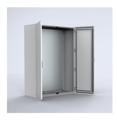
The mild steel double door compact floor standing enclosure range, MKD, is ideal for installation in confined spaces where a single door, when opened, would take up too much space in front of the enclosure. The doors' loading capacity also increases as it is divided over two doors. With a IP 55 protection degree, components inside the enclosure are well protected and makes it well suited for many different applications.
