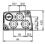
Fig. 13.7: Dimensioned drawing MK 307 connection hood
