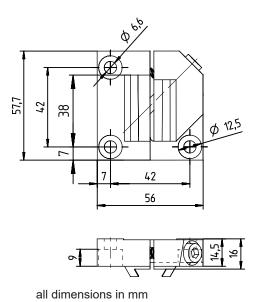
Fig. 13.9: Dimensioned drawing BTU 0300M-W mounting device
