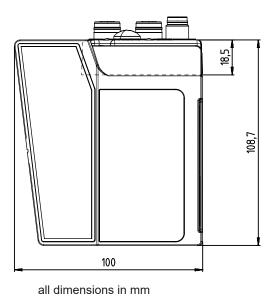
Fig. 13.3: Dimensioned drawing BPS with MS 307 connection hood
