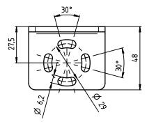
Fig. 13.10: Dimensioned drawing BT 300-W mounting bracket
