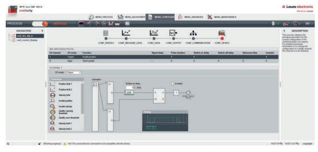
Fig. 9.6: Configuration of the switching outputs
