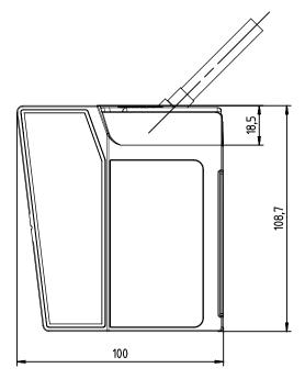
Fig. 13.5: Dimensioned drawing BPS with KB 307 connection hood
