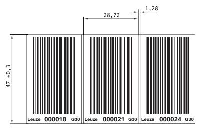
Fig. 13.14: Dimensioned drawing BCB G30 ... bar code tape with 30 mm grid
