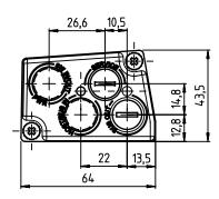
Fig. 13.6: Dimensioned drawing MS 307 connection hood
