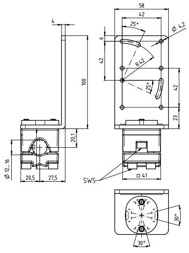
Fig. 13.12: Dimensioned drawing BT 300-1 mounting device
