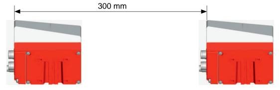
Fig. 6.8: Minimum distance for parallel mounting
