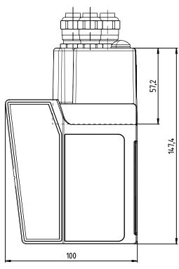
Fig. 13.4: Dimensioned drawing BPS with MK 307 connection hood
