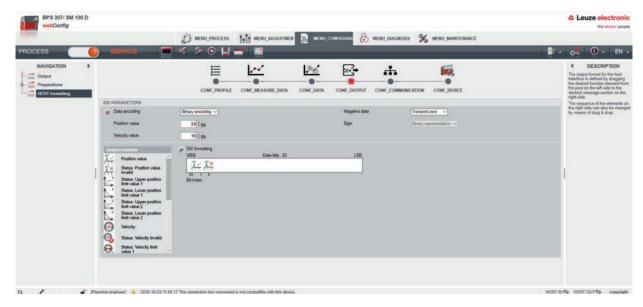
Fig. 9.5: webConfig function *OUTPUT* > *HOST formatting*
