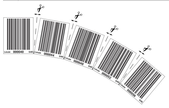
Fig. 6.5: Preparing the bar code tape for use in vertical curves
