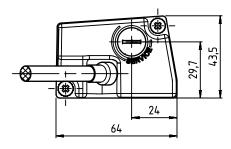
Fig. 13.8: Dimensioned drawing KB 307 connection hood
