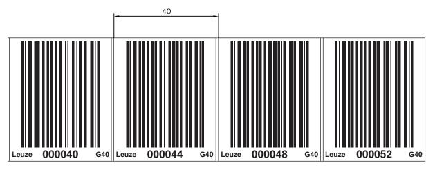
Fig. 11.1: Checking the print result – BCB G40 ...-repair kit (40 mm gird)
