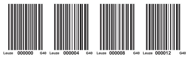
Fig. 16.1: Continuous, 40 mm grid
