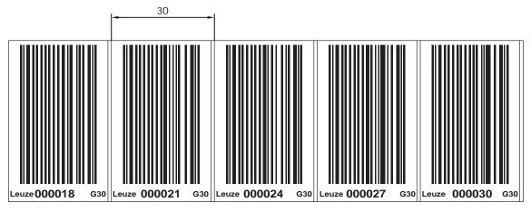
Fig. 11.2: Checking the print result – BCB G30 ...-repair kit (30 mm gird)
