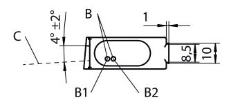
Turning connector, turnable by  $90^\circ$ А
