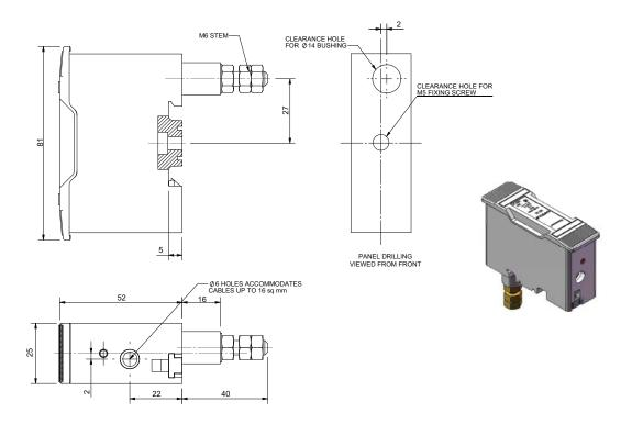
SC32PH-D 32 A, Front/Back stud connected
