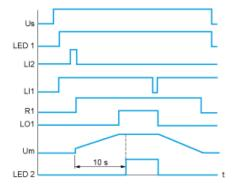
Us : Power supply voltage LED 1Green LED LI2, LLogic inputs R1 : Relay output LO1 :Logic output Um : Motor voltage LED 2/zellow LED
