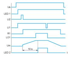
Us : Power supply voltage LED 1Green LED LI2, LL0gic inputs R1 : Relay output LO1 :Logic output Um : Motor voltage LED 2/zellow LED
