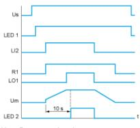
Us : Power supply voltage LED 1Green LED LI2 : Logic input R1 : Relay output LO1 :Logic output LED 2/ ellow LED
