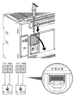
The (-) poles are connected internally.
